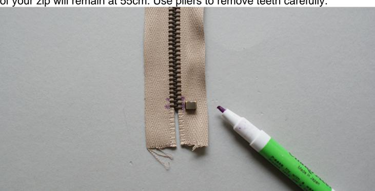
10. Next, we place the Bottom Stop at the bottom'Â of the zip. Place it right below the last bottom tooth. Do not place Bottom Stop diagonally where it would touch both teeth.
