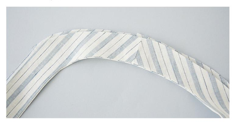
9. Matching the center back seamline of the neckband to the center back notch of the back bodice, start pinning the right side of the outer neckband to the right side of your top. Match the shoulder notches to the shoulder seams and pin along the entire neck opening. Make sure to match the dots on the neckband to the dots on the front bodice.
