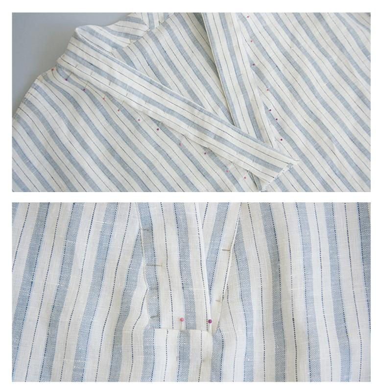
14. Working from the right side, stitch the neckband in place in the ditch of your seam. When you come to the lapped ends at the V-point, pivot your work with the needle still in the fabric and edgestitch across the horizontal edge as close to the folded edge as possible. Stop just in time to pivot again
