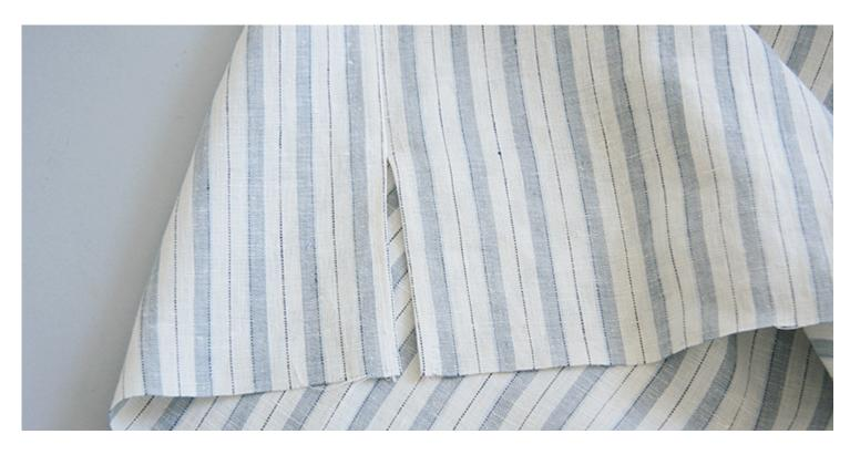
19. Finish the sleeve openings with a rolled hem. Fold your fabric  $\hat{A}^{1/4}_{4}$  at the wrong side and press. Then press another  $\hat{A}^{3/4}_{4}$  and edgestitch in place.
