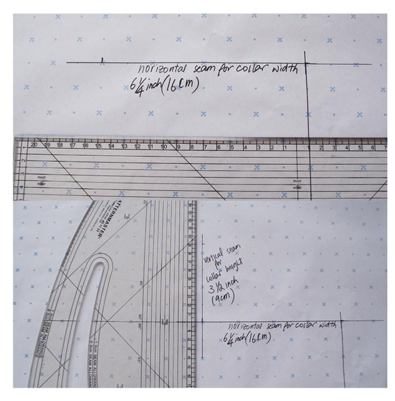
4. For a smooth curve for a collar, use the curve edge of the pattern master or a french curve to help you. Make sure the start point from the centre front seam is flat, and the curve gradually goes up towards the top point, with a smooth curved seam.
