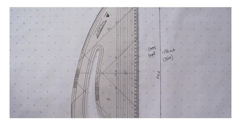
2. As it is at a right angle, you can proceed to draft the bottom seam, as well as the side seam. Both in relation to each other.
